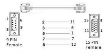
(This cable is used when updating the software or connecting some transceivers (e.g. KENWOOD) via a CAT interface)
