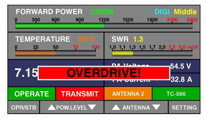
To reset the protection, press the ON/OFF button once. The amplifier will automatically enter "STANDBY" mode. Before continuing to the PA transmission, please remove the cause of activation of the protection control system in accordance with the screen message.
